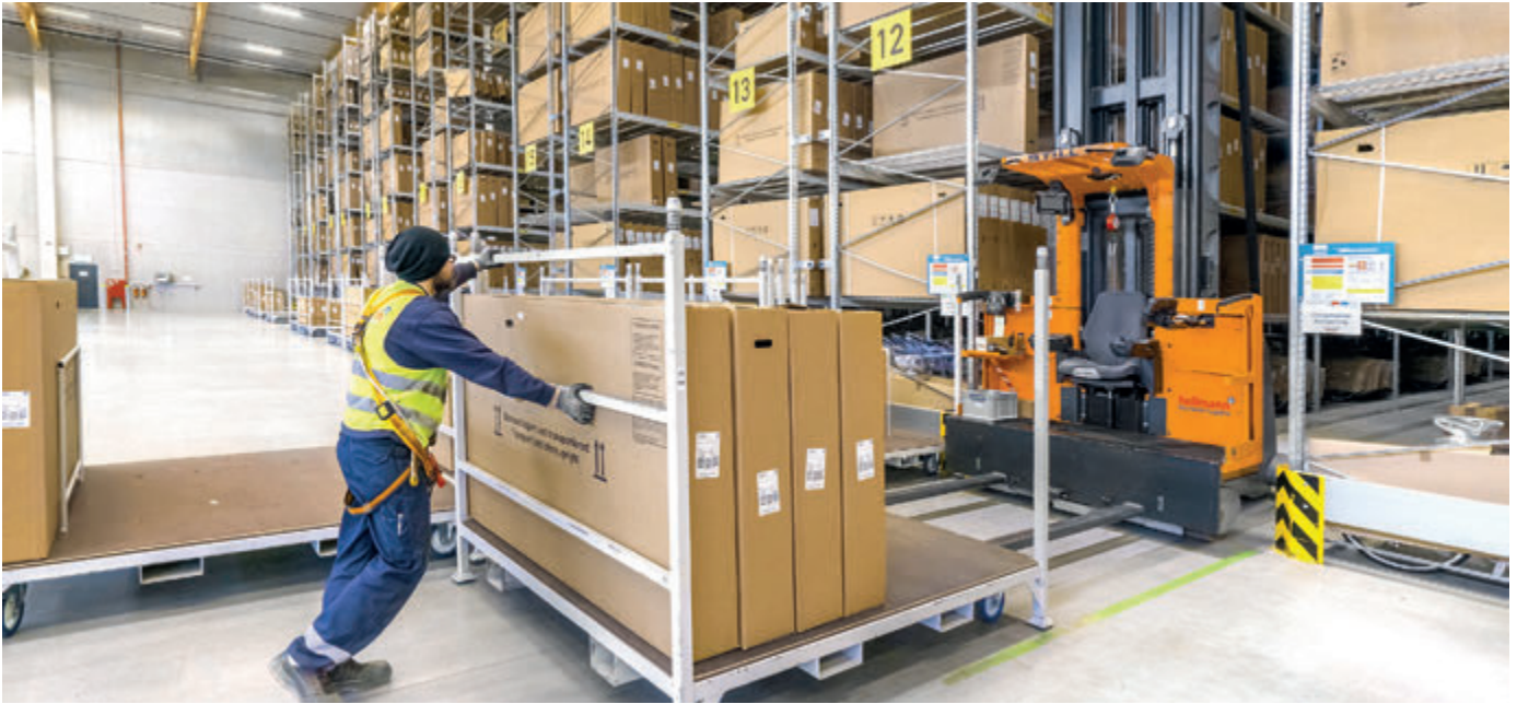
The stake racks can be easily moved manually onto the forks where they automatically lock in position.
