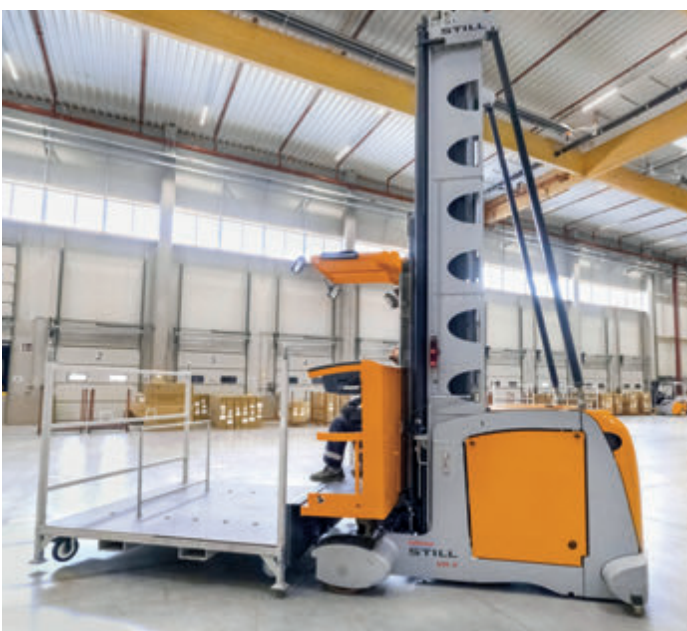
The special design of the VNA trucks allows the use of mobile work platforms, so-called stake racks which are used to order pick bicycles.
