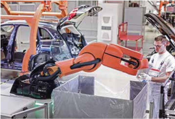
HRC (human-robot collaboration) systems are big news in the world of robotics. This image shows the PART4you system used by car manufacturer Audi: a robotic arm passes the required tools and other items to workers. Photo: AUDI AG
